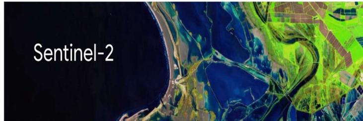
Sentinel-2 (S2) is a wide-swath, high-resolution, multispectral imaging mission with a global 5-day revisit frequency. The S2 Multispectral Instrument (MSI) samples 13 spectral bands: visible and NIR at 10 meters, red edge and SWIR at 20 meters, and atmospheric bands at 60 meters spatial resolution. It provides data suitable for assessing state and change of vegetation, soil, and water cover.
